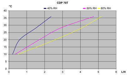
Specific energy consumption (SEC): 0,43 kWh/l at  $28^{\circ}\text{C} \& 60\% \text{ RH}$
